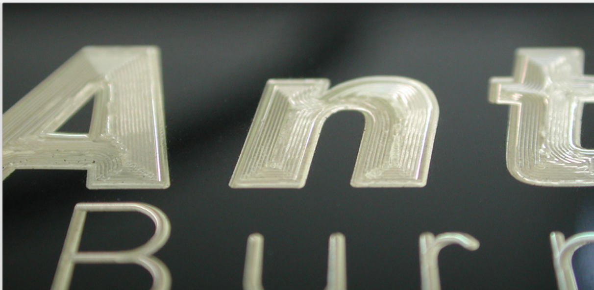
Example of burnishing. Shows single line font and fill font.
