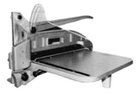
Other than the engraving machines themselves, the most common piece of equipment found in the industry is a shear for cutting material. While there are a variety of sizes and types available, the most popular shear is a twelve inch table model that is relatively inexpensive and capable of handling many of the small plate fabricating requirements in awards and engraving shops.
