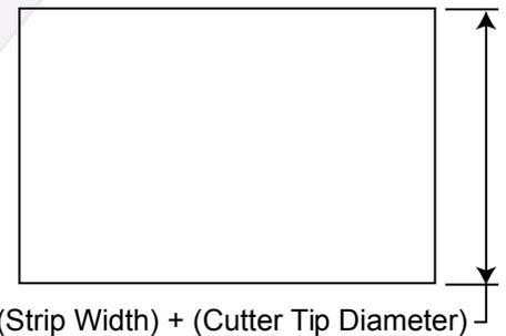
As with the dovetail pattern, it is necessary to factor the cutter tip size when making the calculations. If we are making a strip that is 1.0" x 10" and we are using a profiler with a .030" tip, we would add .030" to each dimension. The result would be a rectangle measuring 1.030" x 10.030". When making the strips, we are concerned with the inside of the cut, so the cutter width is added instead of being subtracted.
