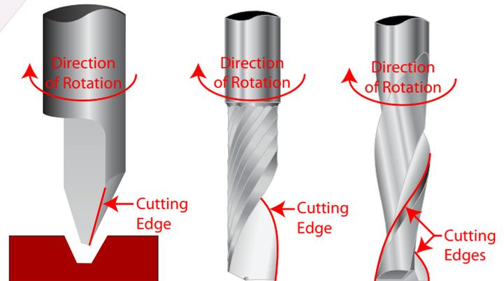
**Cutters can be classified as half-rounds or quarter-rounds. This refers to how the blank carbide shafts are split during the manufacturing process.**
